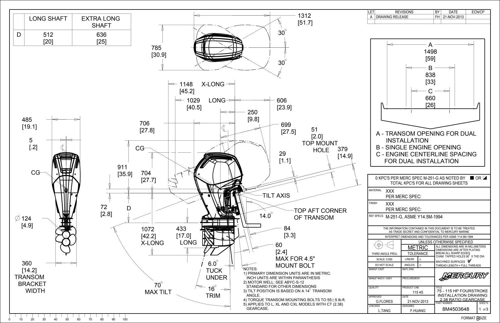
NOTES: 1. STATIC WATERLINE MUST BE BELOW THE IDLE RELIEF OPENING (LOCATED AT REAR OF OUTBOARD) WHEN OUTBOARD IS AT FULL TUCK. INCREASE OUTBOARD MOUNTING HEIGHT OR ADJUST BOAT LOAD IF IDLE RELIEF IS BELOW STATIC WATERLINE AT FULL TUCK.
